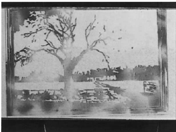
Fig. 9. A picture of a village printed on the slide glass substrate surface by LIPAA.
